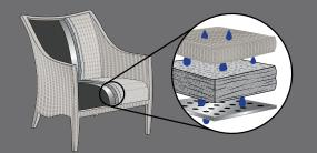
Perforated aluminum frame is wrapped in quick-dry reticulated foam upholstered in N-Dura™ resin wicker.
